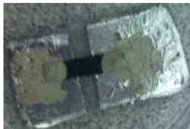
Figure 2. Photosensor of a sample of nanocomposite with graphene oxide.
